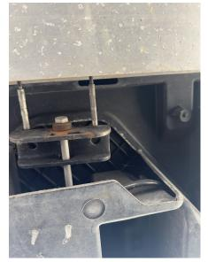
Assemble the master cylinder mount as shown.
