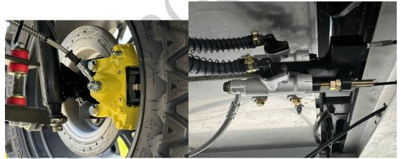
A 2" access hole may be drilled to cleanly pass the brake reservoirs up through the seat area. (most electric carts) You should be able to completely remove the masters, reservoirs, calipers and lines without disassembling any of the plumbing.
