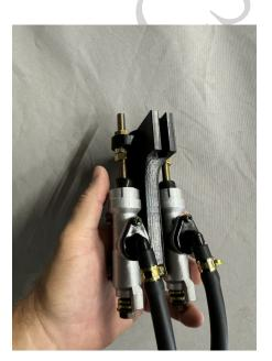
We recommend lengthening the typical master cylinder reservoir hose up to 36" before install.
