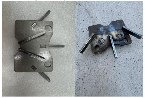
Clamp the bracket against the rotor as shown. Fully seat the narrow concave side against the axle. Make sure the caliper bracket is parallel to the rotor and spaced properly using the press in gussets.
